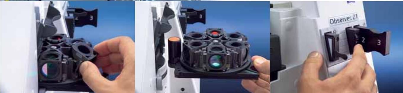
*Reflector turret: in a matter of seconds, filter sets are now replaced without removing the reflector turret.*
